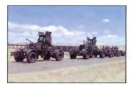
Husky/Meerkat: Mine/IED Detection/Detonation Vehicle Requirement: 70 On Hand: 68 Delivery Schedule: 1/month Requested an additional 60 vehicles
